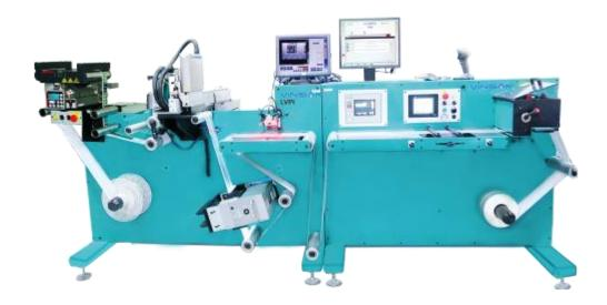
When it comes to printing personalized security labels with fully variable information, or frequently changing print the VINSAK LVPI is the unique solution. With installed VINSAK VIS 1200, UV drying unit and camera on the VINSAK rewinder, this makes possible to print personalized data digitally onto various offset papers, coated papers, gloss papers, PET, BOPP including holographic substrate's etc. The main benefits of having LVPI are:
